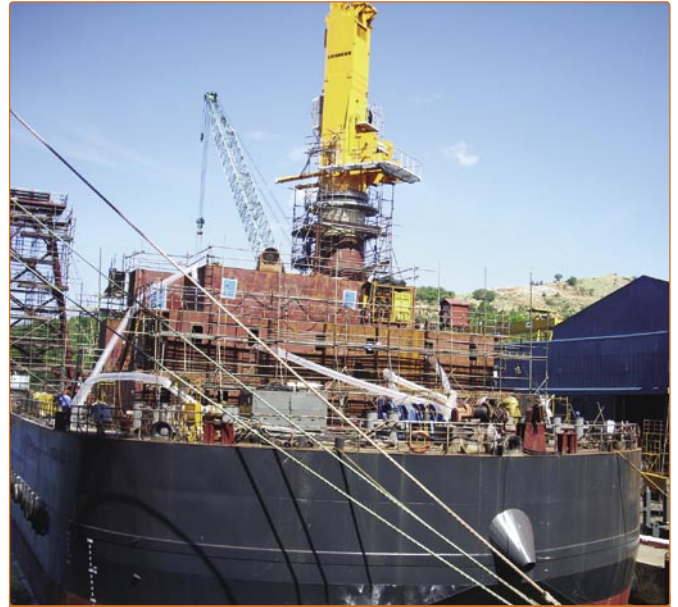
The Logmarin floating crane has been designed for both harbour and open water operations, and is equipped with combined 'Rolling Damping Systems'.
